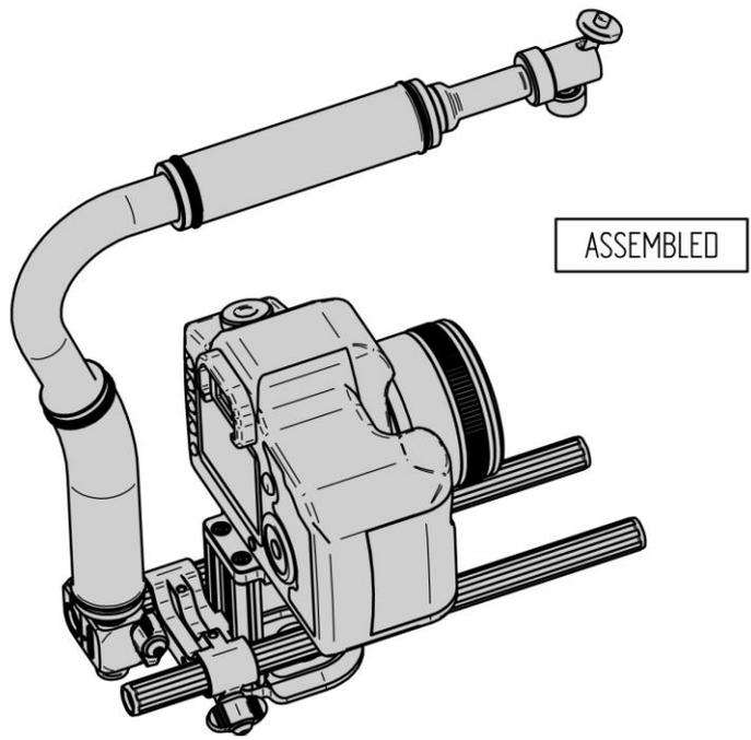
**BEFORE USE CHECK IF THE CLAMPS ARE TIGHTENED**
